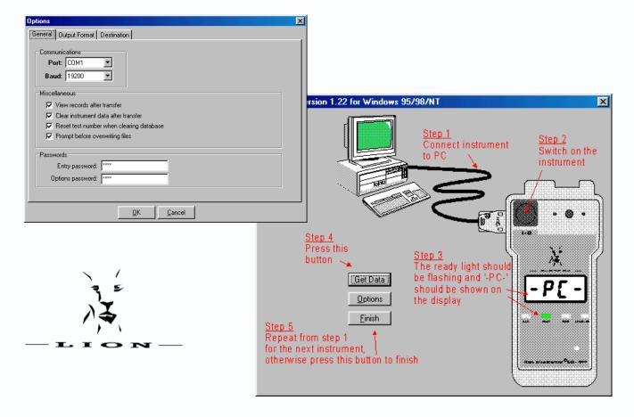
Each time a lion alcolmeter® 400 tests a subject's breath, data is stored in its memory. This data may simply be the alcohol reading, with date and time; or it may, if the instrument has data logging capabilities, include the test location and reason codes, the identity number of the operator, and the sex of the subject as well.
