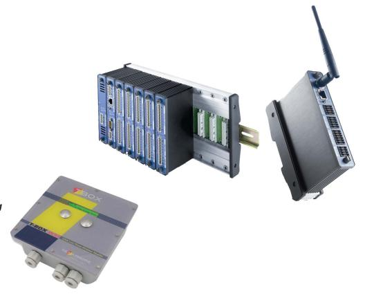
Each T-BOX RTU is an allin-one package that brings an integral Web server, push communications, and reporting via email and SMS text messaging to monitoring and control applications. Semaphore's innovative technology enables real-time access, anywhere, with a mobile phone, PC or PDA to create a highly costeffective solution.
