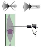
The flue gas must be able to flow freely past the thermocouple.
